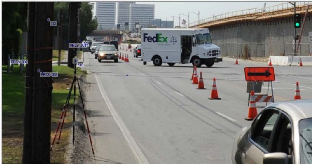
Figure 6: Reference targets along roadside
