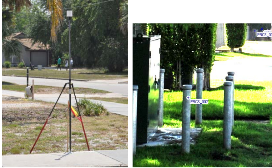
Figure 2: Typical LiDAR reference targets
