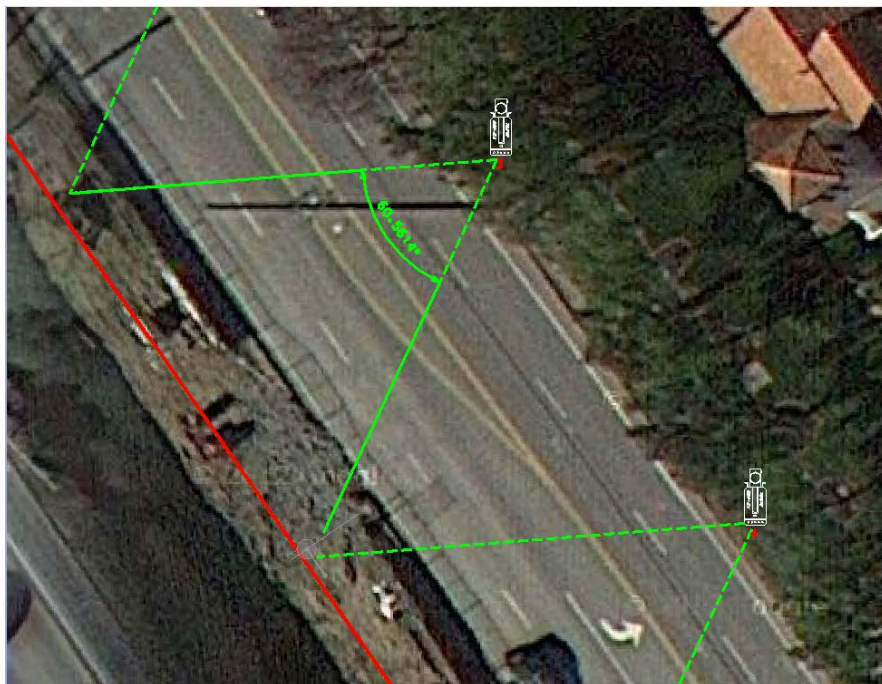
Figure 37: Top View Scanner Position-Wall Alignment (TopoDOT™)
